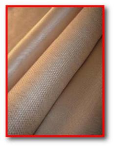
This premium grade high temperature and heat resistant woven fiberglass cloth is heat treated to remove organics, set the weave dimensionally and reduce fray and loose fibers. Meets MIL-C-20079 (type I, Class 9) and US Coast Guard 164.009.
