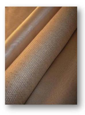
High temperature, heat and flame resistant thermal insulating fiberglass fabric fabricated from high quality type E fiberglass that will not burn and will withstand continuous exposure to temperatures of 1000°F / 520°C. It is used to protect equipment, wires, cables, hoses, tubing and pipes. This high temperature fabric provides thermal insulation and personnel protection.
