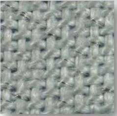
This material resists most acids and alkalis and is unaffected by most bleaches and solvents. It is highly flexible and conformable.
