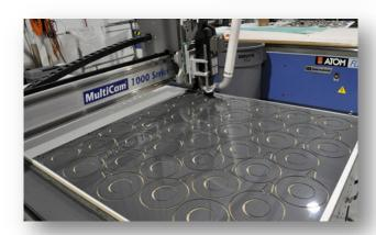
OSCILLATING KNIFE CNC CUTTER
