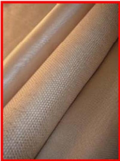
This premium grade high temperature and heat resistant woven fiberglass cloth is heat treated to remove organics, set the weave dimensionally and reduce fray and loose fibers. Meets MIL-C-20079 (type I, Class 9) and US Coast Guard 164.009.
