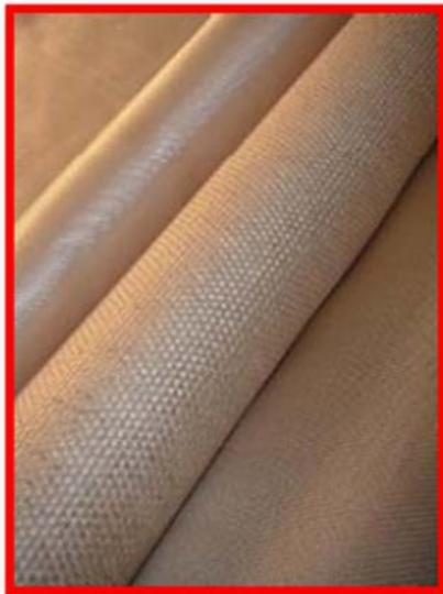
This high temperature, heat and flame resistant thermal insulating vermiculite coated fiberglass fabric will withstand temperatures of 1500°F / 815°C continuous exposure. The base High Temperature fiberglass fabric is fabricated from high quality type E fiberglass that will not burn. The fabric is then coated with a vermiculite dispersant.
