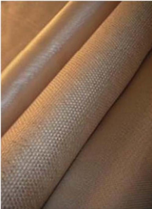
This high temperature fabric is a non-asbestos replacement fabric, made from high temperature, heat & flame resistant fiberglass fabric with an interwoven stainless steel wire which accounts for 10% of the fabric's weight. If you look carefully at the photo, you can see the stainless wires.
