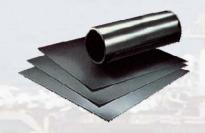
Flexible graphite sheet is made from exfoliated graphite flake, which is compressed into foil by a carefully controlled calendaring process. In this process, the expanded flake particles are mechanically locked together without the use of fibers, binders or other additives. The Flexible Graphite sheet is laminated with an adhesive bond on both sides of a .002" thick 316 stainless steel foil insert. Used where high performance and handle ability are important.
