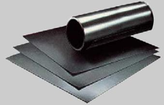
**Flexible Graphite Sheet** is made from exfoliated graphite flake, which is compressed into foil by a carefully controlled calendaring process. In this process, the expanded flake particles are mechanically locked together without the use of fibers, binders or other additives.
