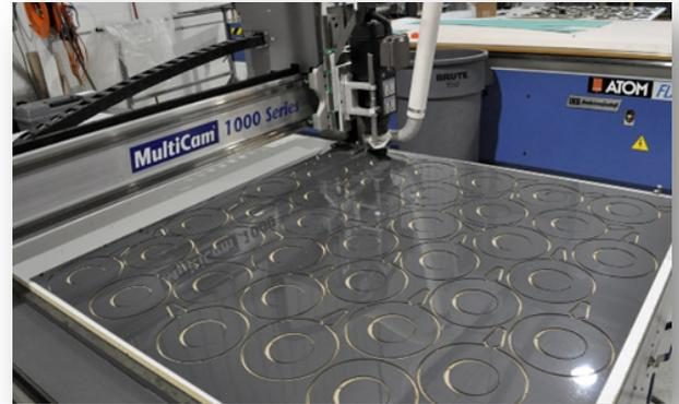
**OSCILLATING KNIFE CNC CUTTER
