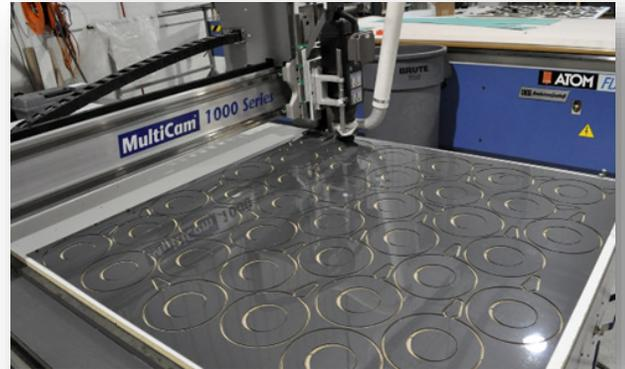
**OSCILLATING KNIFE CNC CUTTER
