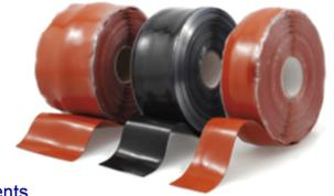
The tape has no adhesive, but sticks to itself (self-fuses or self amalgamating) when stretched and wrapped onto it self. The tapes starts curing within minutes, and after several hours cannot be unwound or removed without using a sharp knife or blade. This tape makes a waterproof, weatherproof and air-tight protection.
