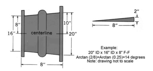
The degree of taper should not exceed 25° where a taper is more than 15°, a filled arch is recommended. Where a filled arch is utilized, the available movement will be decreased 50% from that of an open arch.
